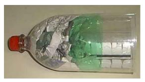
4. Place two liter bottle (pressure vessel) into top half. Try to make bottles straight. Use little pieces of tape to secure bottles.
