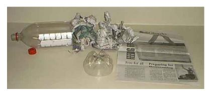
3. Push bottom half of two liter bottle upside down into top half – to keep ballast in place.
